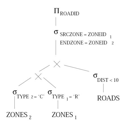
Figure 7: Query tree after the selections have been pushed down.
