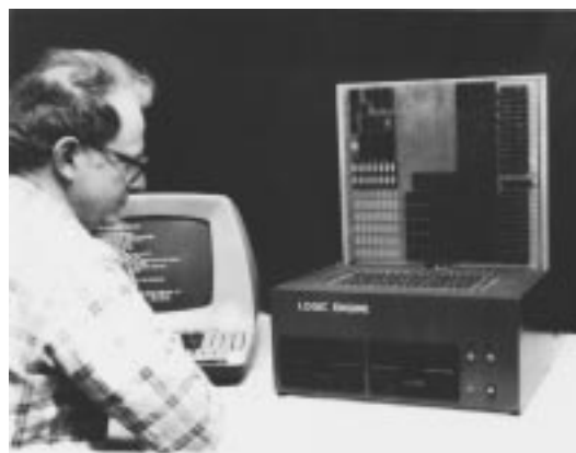
Photo 3. This photograph shows the predecessor to the current Logic Engine, used between 1980 and 1990. It’s backpanel is the project area. The base unit holds a primitive M6809 based workstation.
