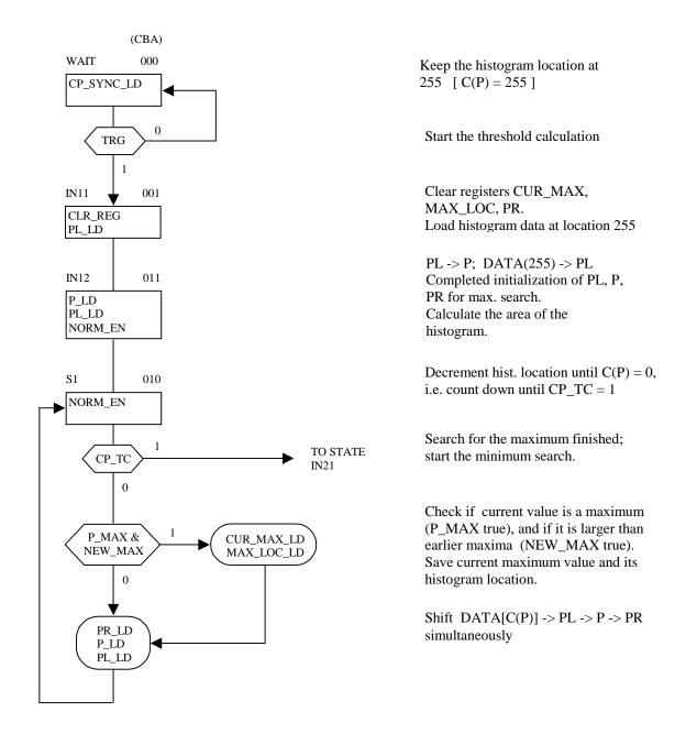
Picture 25: Control ASM for the histogram/threshold calculation, p.1
