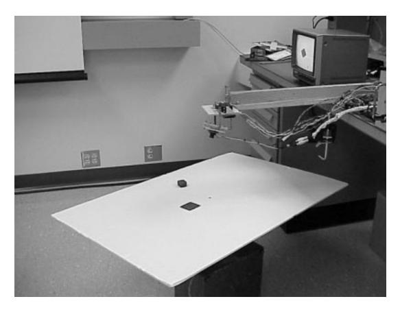
Picture 11: Laboratory set-up for the tracking-speed measurements
