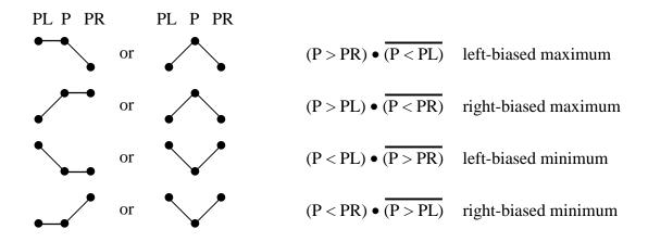
We use the left-biased comparisons. Current extremes are latched into registers CUR\_MIN and CUR\_MAX. Since we are interested in the global extremes, locally found extremal values must be compared with current largest/smallest values. All the comparison logic is contained in the schematic HIST\_MINMAX.
