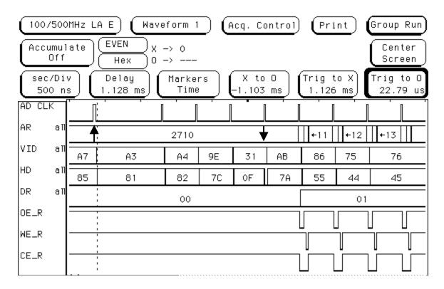
Picture 17: A/D pipeline delay
