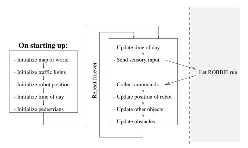
Figure 3.4: Simulator's process
