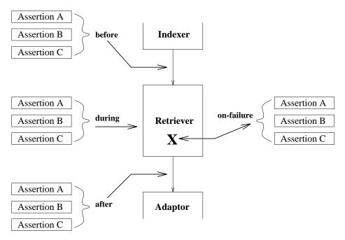
Figure 6.1: Assertions refer to points in processing: before, during, after, and on-failure.
