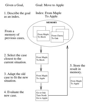
Figure 2.1: A typical case-based planner
