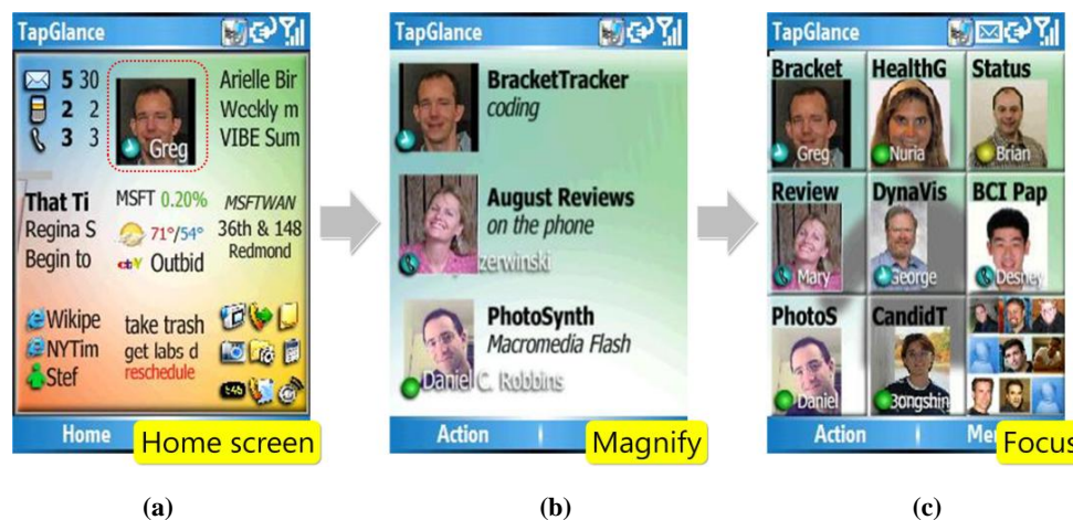
Figure 2. The TapGlance prototype shows glanceable information on the main screen (a). In the magnify view (b) detailed awareness information is shown for a small group of people. In the focus view (c) users can see high-level status information for several people which they can use to drill down for additional information.
