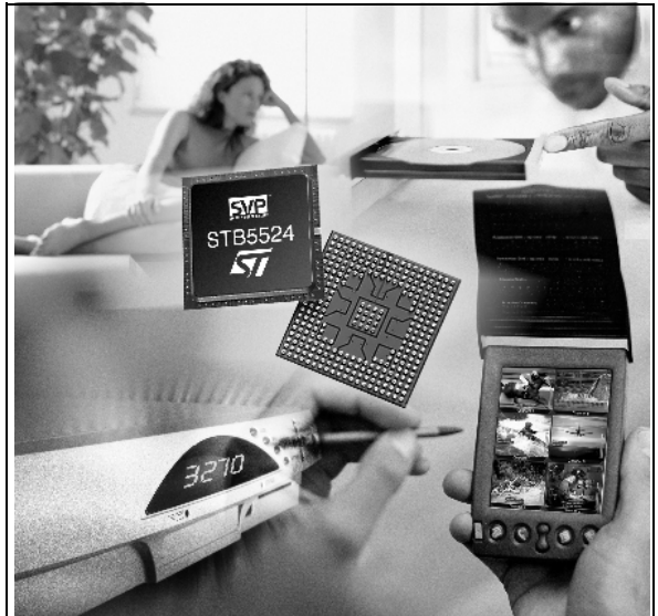
Figure 1. Package (27 x 27 PGBGA 416, 1 mm pitch)
