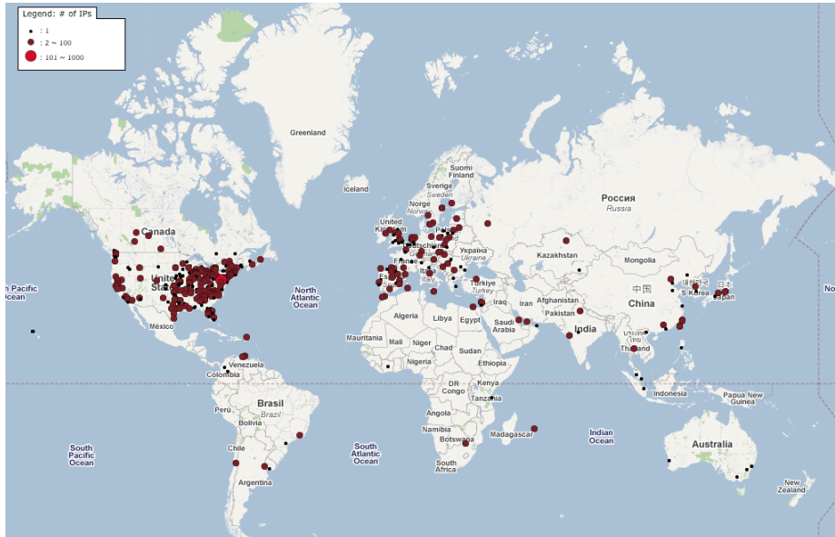
Fig. 14. Geographical distribution of IP addresses of JavaScript-delivery hosts. The size of icons for each point is proportional to the number of IP addresses for that location.
