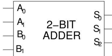
Here is a design to implement the adder, consisting of one equation for each bit of output, plus one additional equation defining a local subterm, the carry-bit from the 1s' place. ( $\oplus$  stands for the *exclusive-or function*,  $\wedge$  for “and” and  $\vee$  for “or”):
