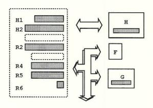
abstraction, such as memory or queue, is encapsulated as a process entity. Such transformations often introduce of new registers—in the diagram, H1 and H2 result when R1 is incorporated with H. For example, a factored memory would leave residual address and content registers.
