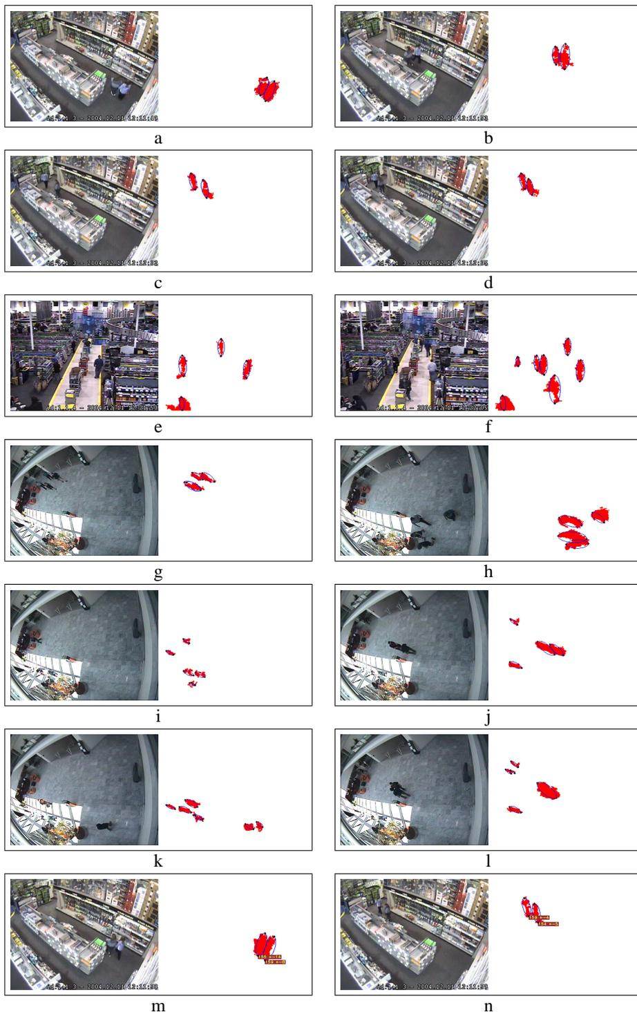
Figure 7: (a) - (l) Head candidates from test frames. Left image is the original frame. On the right image red represents foreground mask, small black dots indicate the locations of  $T_i$  and  $B_i$ ; blue ellipses are fitted with  $T_i B_i$  as the major axis; (m) and (n) Height detection: brown plates contain height mean and variance for each ellipse
