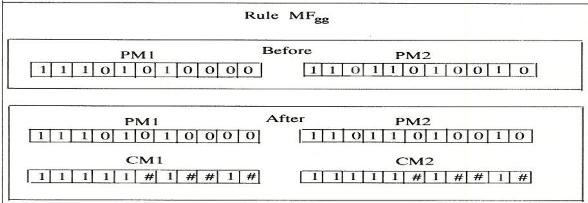
Figure 9: Mask rule MF_{gg} : Example of mask propagation when both C1 and C2 are good
