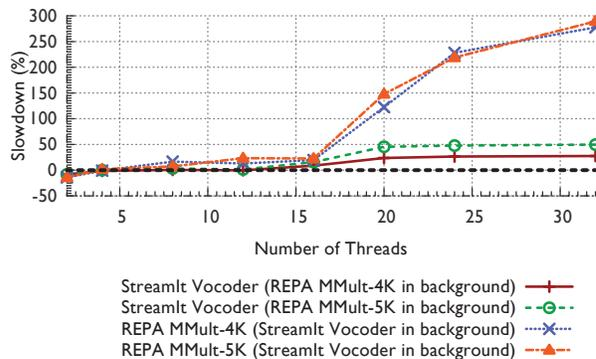
**Figure 4.** Running the StreamIt Vocoder benchmark in parallel with gang-scheduled, parallel matrix multiplication (REPA). For up to 16 cores, both benchmarks execute in isolation resulting in a negligible slowdown.
