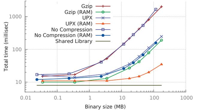
**Figure 2.** Load and execute overhead for a *hello-world* binary of different sizes. Embedded as a Haskell byte array with (1) Gzip compression, or (2) as a UPX packed executable, or with (3) no compression at all.
