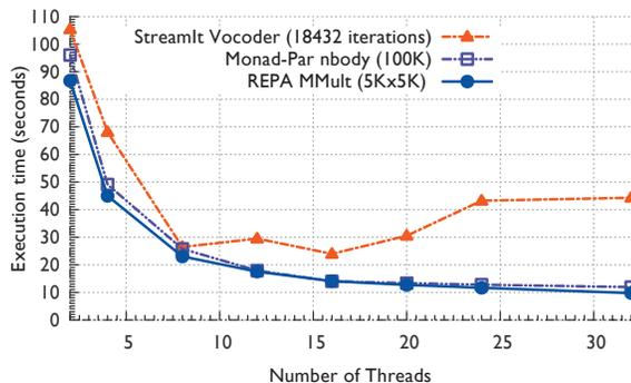
**Figure 3.** Baseline performance of a sequential Haskell program with synchronous calls to (1) the StreamIt Vocoder benchmark, (2) the Monad-Par nbody benchmark and (3) REPA matrix multiplication benchmark. Thread settings  $> 16$  represent hyperthreading. Results are from the streamit-3.0 development branch, with a 16-core Intel E5-2670, and `strc -O2 --smp`.
