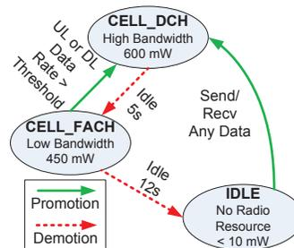
**Figure 1: RRC State Machine of a large UMTS carrier in the U.S. The radio power consumption was measured by a Monsoon power monitor [3] on a Google Nexus One (HTC Passion) smartphone. More details can be found in [17].**
